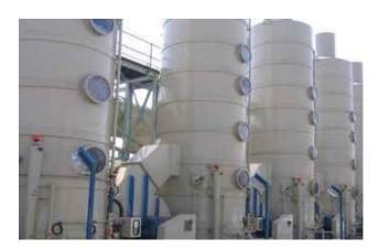
PP is the ideal material for use in pickling plants, the chemical industry, and also for extremely aggressive waste water, as chemicals are used at high temperatures in these areas. The AGRU product range includes various PP polymer types:
