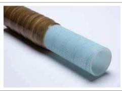
The PVDF HV-Liner from AGRU is an economical alternative to traditional fabric backed pipe. The surface-treated PVDF pipe has a three-dimensional surface structure that provides for optimal bonding with the GRP pipe. The piping systems are available in PVDF, PVDF-FLEX, and PVDF-el. The pipes can be produced in diameters from 20 – 355 mm.
