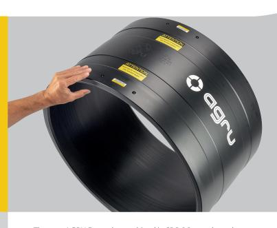
The new AGRU E-coupler machined in SDR 26 completes the system and opens new application fields. Leightweight and thus easy to handle, the SDR 26 E-coupler made from PE 100-RC requires short welding times **without pre-heating.** Ovalities of the components to be welded as well as big annular gaps are compensated widely to provide a perfect welding result. If for sewage, industrial applications or fishfarming, the AGRU SDR 26 E-coupler provides the perfect fit.
