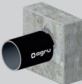
The AGRU Flex Restraint is a flexible bar for electro-socket welding onto PE 100 / PE 100-RC pressure pipes. This way, a rigid system by fixed points can be created that absorbs high forces to prevent axial movement.
